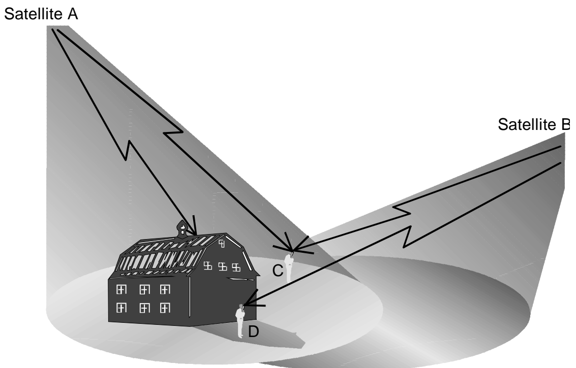
Figure 43 Downlink carriers to mobile terminals in overlapping satellite coverage areas, one in a shadow
